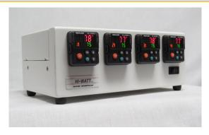
The Quad series offers four zones of control in one package. The Quad series are fitted with Watlow Series EZ Zone PM controls. Each zone utilizes a solid state relay for longer heater life and a lower cost than other power switching devices. The heater output connectors can be ordered as either an Amp Mate-n-Lok or twist and lock connector. Control Consoles are also available are a single and dual zone models. Custom options are also available.
