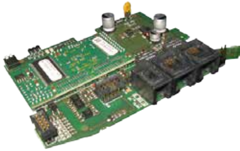
Figure 35 Port2: Modbus RTU / Ethernet IP or Modbus RTU/EtherCAT or Modbus RTU / ProfiNET Interfaces
