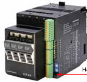
Figure 35 Port2: Modbus RTU / Ethernet IP or Modbus RTU/EtherCAT or Modbus RTU / ProfiNET Interfaces
